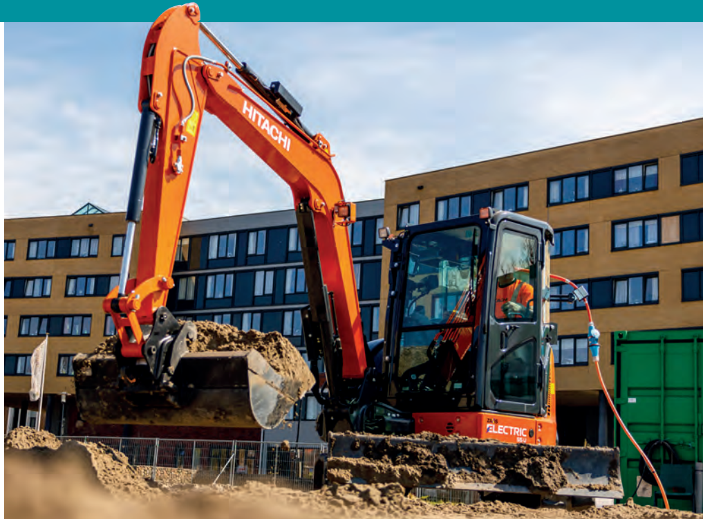
According to Hitachi, the ZX55U-6EB has been designed to provide similar levels of performance as diesel alternatives. PHOTO: HITACHI
