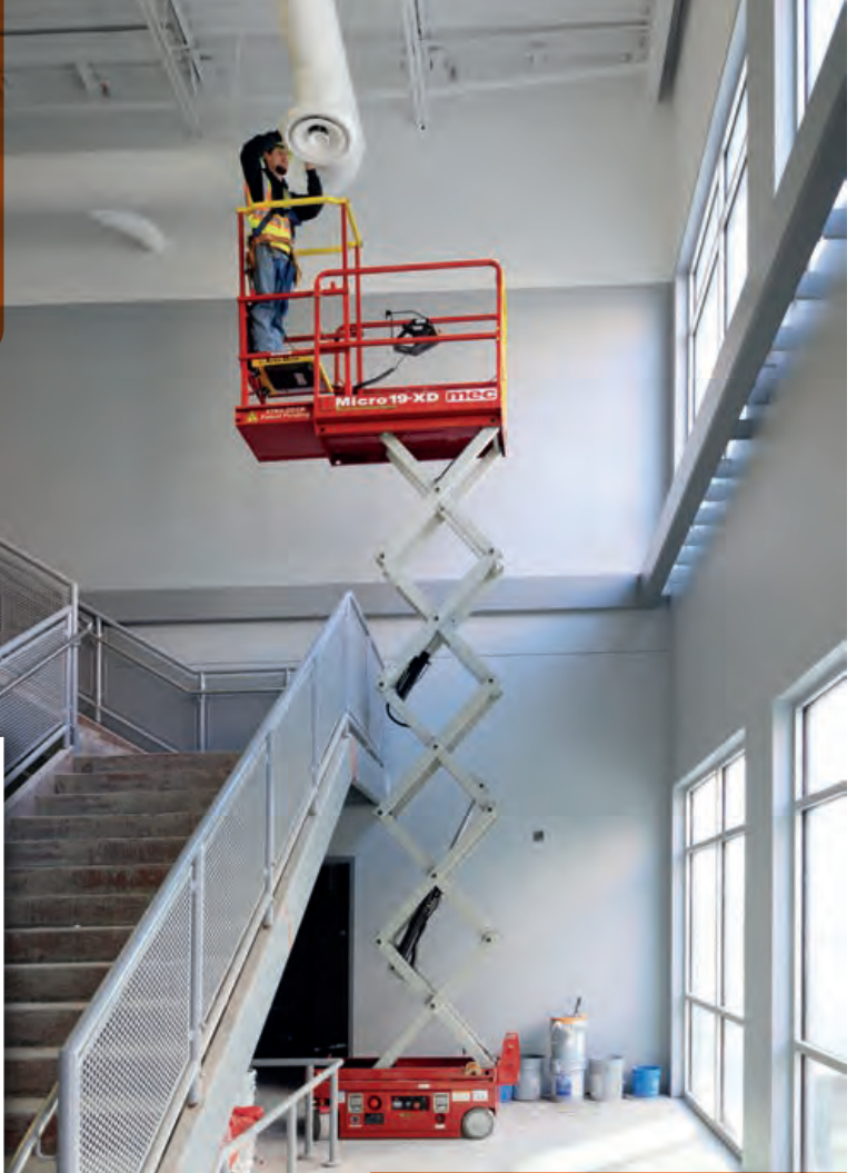
MEC Aerial Work Platform's Micro19-XD micro scissor lift.
