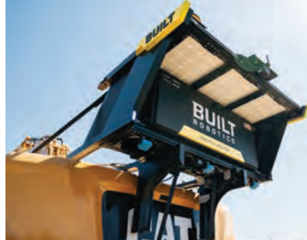
Built Robotics' Exosystem on the back of a Caterpillar machine. The Exosystem is installed to enable the machines to operate autonomously. It includes an all-weather enclosure, proximity radar, 360 degree cameras, GPS and a liquid-cooled computer. PHOTO: BUILT ROBOTICS
