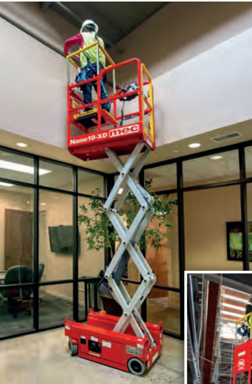
MEC Aerial Work Platform's NANO10-XD micro scissor lift.
