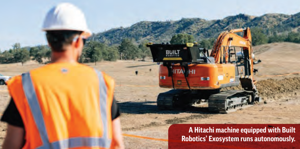
Built Robotics' Exosystem on the back of a Caterpillar machine. The Exosystem is installed to enable the machines to operate autonomously. It includes an all-weather enclosure, proximity radar, 360 degree cameras, GPS and a liquid-cooled computer. PHOTO: BUILT ROBOTICS
