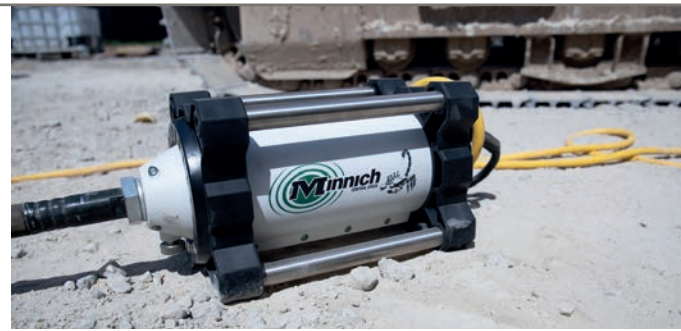
Minnich has a Control Speed Vibrator (CSV) with which contractors can choose the speed they want the vibrator to run based on the workability of the concrete
