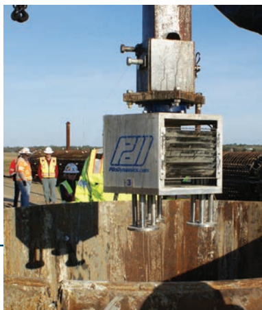
The Shaft Quantitative Inspection Device, also known as SQUID
