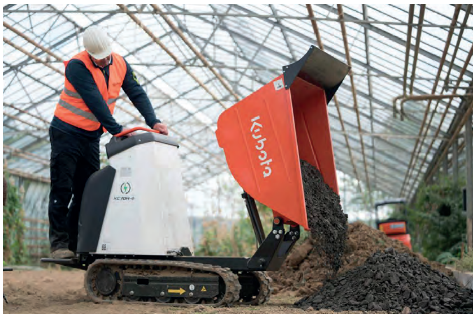
The Kubota KC70H-4e electric tracked dumper – a single 3-hour charge powers a day's work.
