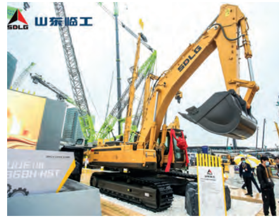
China-based OEM Shandong Lingong, (SDLG) the E660F-Ex electric excavator, which uses lithium battery technology.
