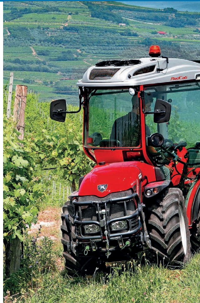
The Tora Series tractors by Antonio Carraro have Stage-5 engines but kept almost the same dimensions of previous models. The reversible Tora tractors can be equipped with the new RGS reversible drive system on a rotating control tower that rotates 180° to invert the drive direction.
