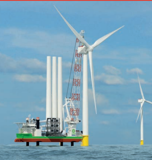
Sea Installer will get a major crane upgrade raising capacity from 900 to 1,600 tonnes
