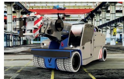
Manitex Valla's new V210R can be controlled via radio remote control
