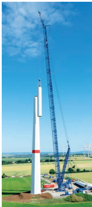
Liebherr has two new cranes, the 700 tonne LR 1700-1.0, pictured, and the 40 tonne LTR 1040
