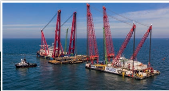
Scaldis completed a simultaneous and synchronised 5,000 tonne lift with its vessels Rambiz and Gulliver
