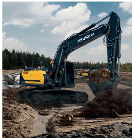
Hyundai's HX210AL 22 tonne crawler excavator carries the new A series livery, as well as machine control and machine guidance features
