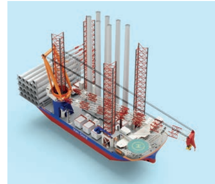
Artist’s impression of the new Van Oord offshore installation vessel for 20 MW turbines with 3,000 tonne Huisman leg encircling crane
