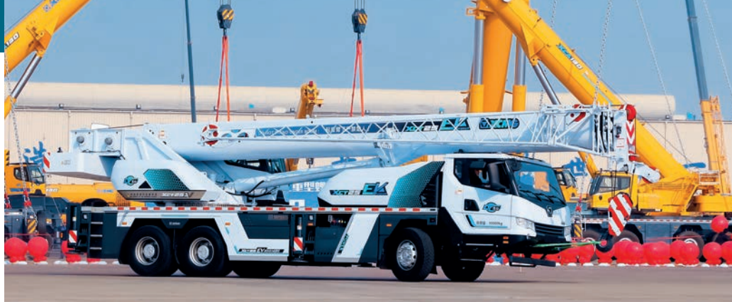
The new XCT25 EV truck crane from XCMG at its launch in November. It is a 25 tonner with hybrid powertrain
