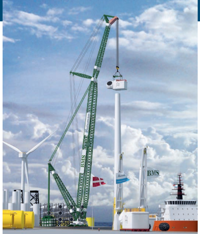
How the new 3,000 tonne capacity Huisman Ringer Crane will look in BMS colours at work lifting turbine components on a quayside
