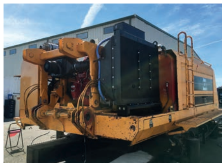
Replacing the engine in this Manitowoc 888 crawler allowed it to be brought up to current exhaust emission specifications
