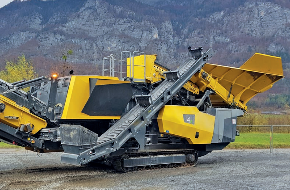
The new mobile I4e reversible impact crusher from Keestrack is designed for the recycling of building materials
