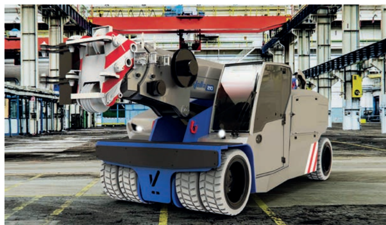
Manitex Valla's new electric V210R can be controlled via radio remote control or directly from its cabin
