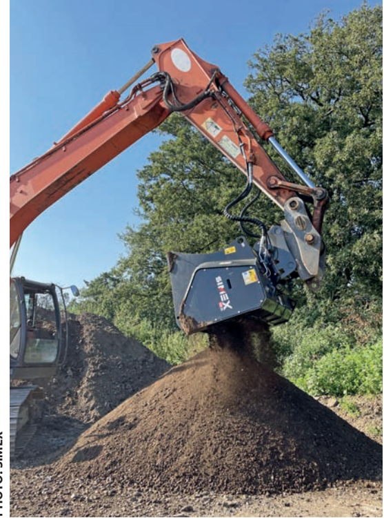
Simex's VSE screening buckets - for excavators of between 8 and 48 tonnes
