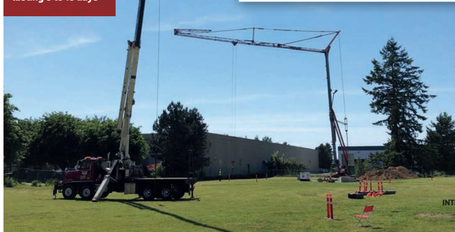
Self erecting tower crane and stiff boom crane students training on at Bigfoot's Abbotsford BC Training Centre. Both are full certification programmes lasting 8 to 15 days
