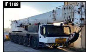
GROVE GMK 5130-1 Year 2006 60.0 meter boom + 8 meter extension + 18.0 meter swingaway with hydraulic offset
