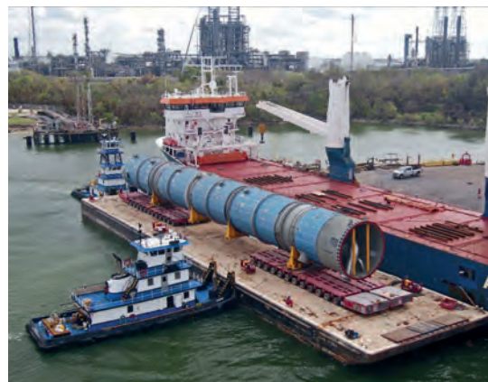
The 972,912 pound deisobutanizer is placed on barge-mounted Mammoet SPMT for offloading
