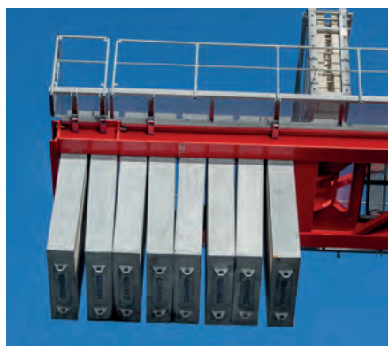
Galvanised steel frames on each block
