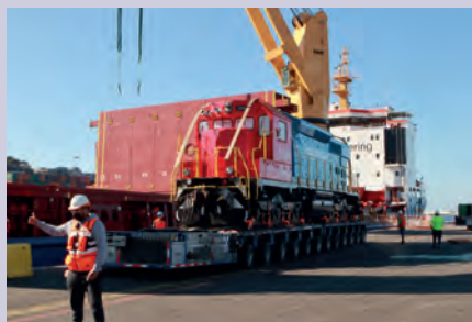
The railway locomotives were removed sequentially using Engineered Rigging SPMT
