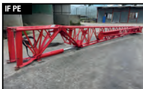
GROVE GMK 5130-2 & 5110-1 Hydraulic swingaway including 2x boom inserts
