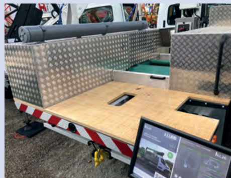
Klubb's new prototype flat bed, made of bamboo composite.
