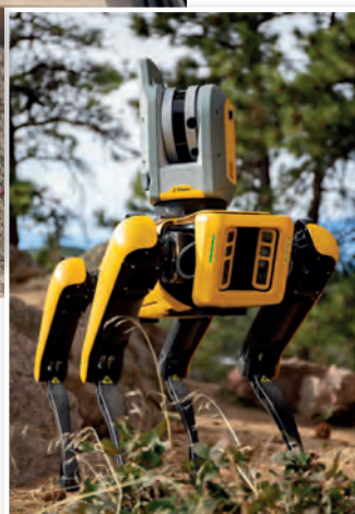
BOSTON DYNAMICS' SPOT ROBOT WITH TRIMBLE X7 3D SCANNING SYSTEM
