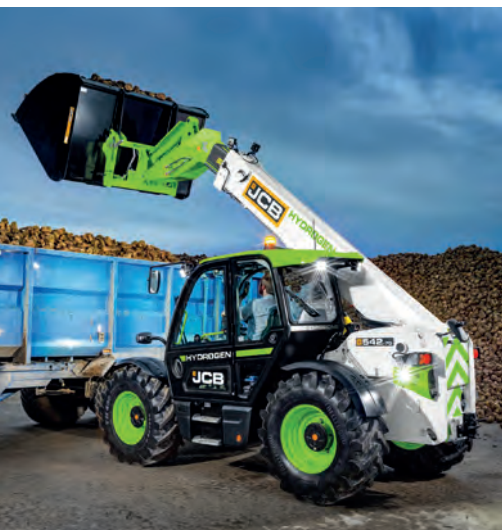
JCB IS USING HYDROGEN COMBUSTION ENGINES IN WORKING TEST MODELS OF ITS 3CX BACKHOE-LOADER AND 542-70 LOADALL TELEHANDLER.
