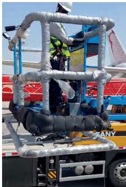
The Dayim team has developed a purpose built solution for the aviation industry, enhancing aircraft maintenance safety by preventing accidental collisions of platform baskets with aircraft during maintenance.
