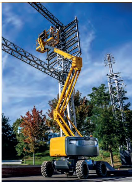
Haulotte's latest Pulseo, the HA16 E, has an interchangeable range extender.
