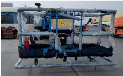
The Dayim team has developed a purpose built solution for the aviation industry, enhancing aircraft maintenance safety by preventing accidental collisions of platform baskets with aircraft during maintenance.
