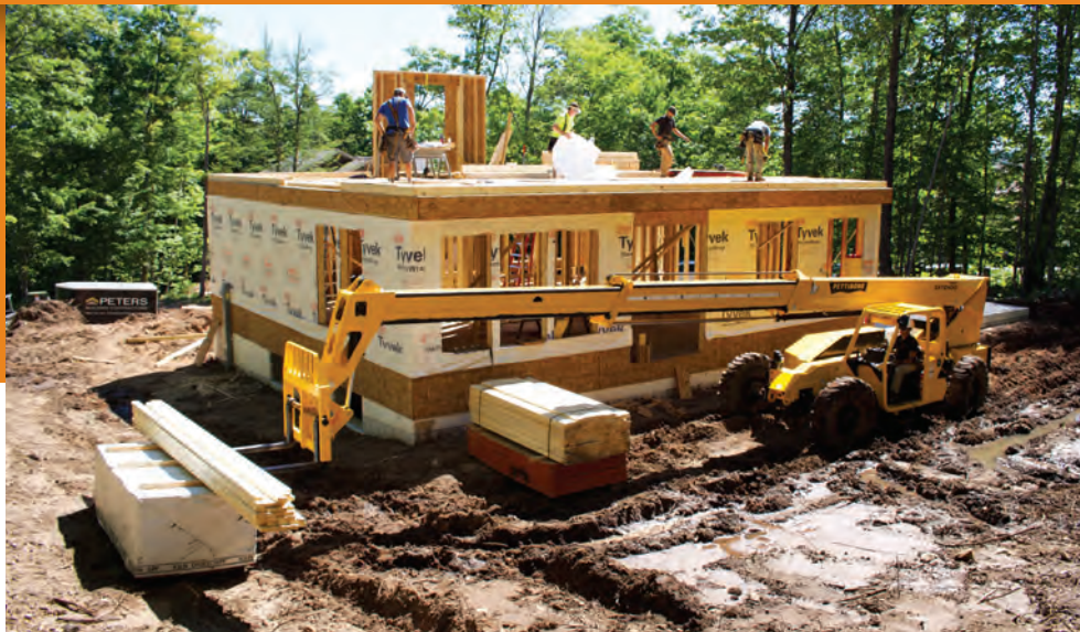
The Extendo 1536X has a maximum load capacity of 6,804kg. PHOTO: PETTIBONE
