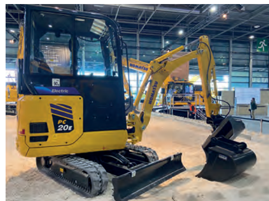
The PC20e is powered by a 11.9kW battery that can last up to eight hours.
