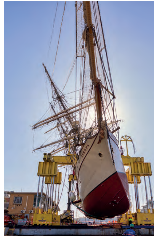
Using four hydraulic gantries and a strand jack system, the Vanguard team designed a bespoke solution to upright the Europa ship.
