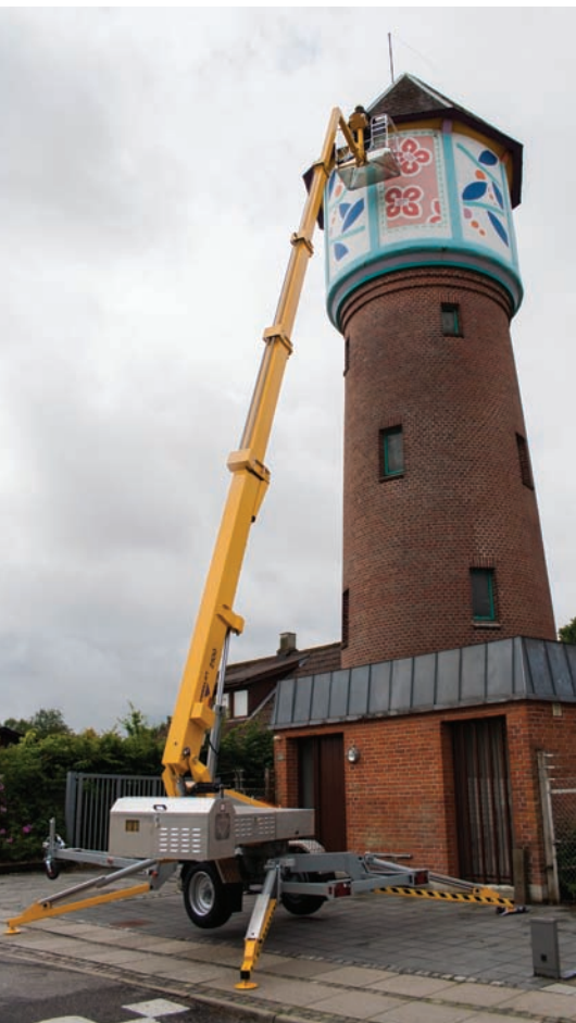
A TSJ35 wheeled Palazzani with outriggers.
