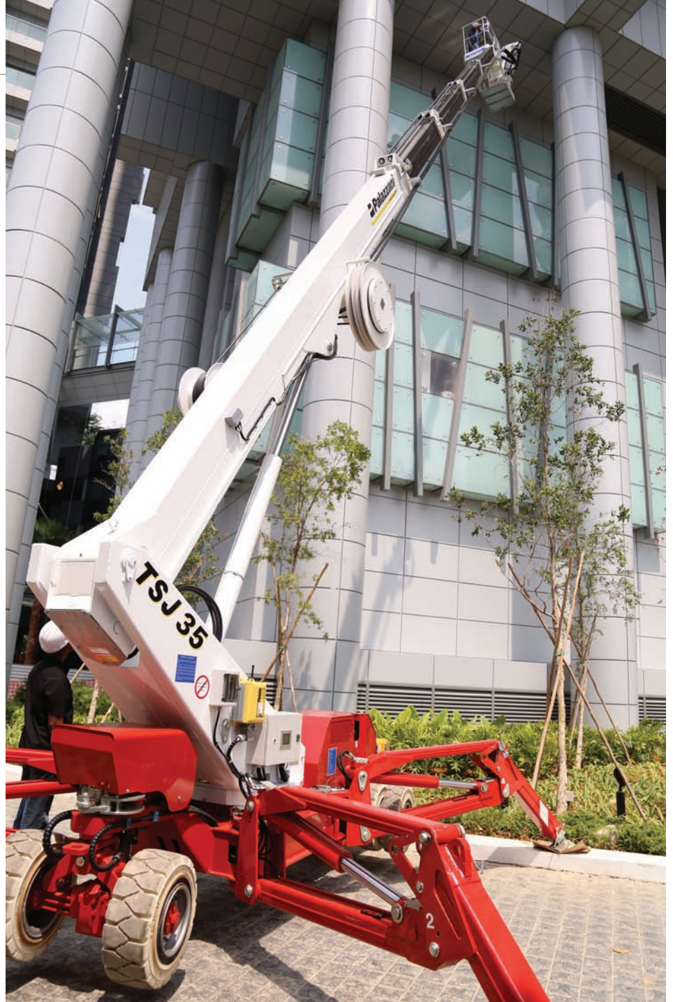
A TSJ35 wheeled Palazzani with outriggers.
