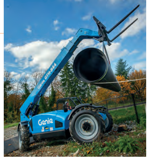
The Genie GTH-844 telehandler has a 8,000lb capacity
