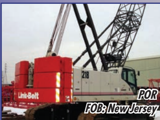
2007 Link-Belt 218 HSL 110-ton, 150' main boom, "ABC" Ctws Block/Ball, diesel engine. POR
