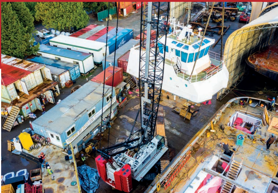
The first major project for the new Link-Belt 298 Series 2 crawler was lifting a 125,000-pound pilot house for a new hybrid tractor tugboat.
