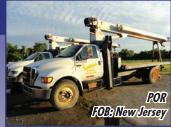
2005 Manitex 1770C 17- Ton, Ford F750 210 HP CAT, 20' wood deck, 23' 1-piece jib
