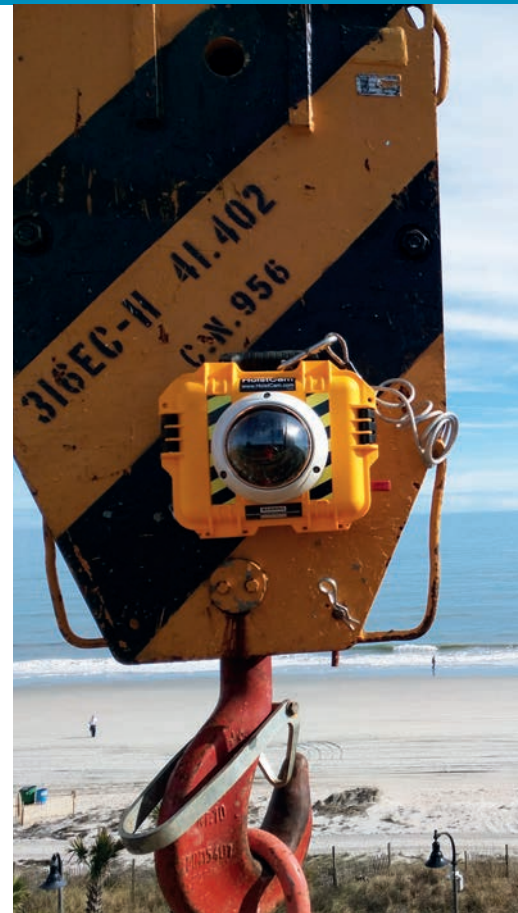
Crane cameras give operators a closer look.
