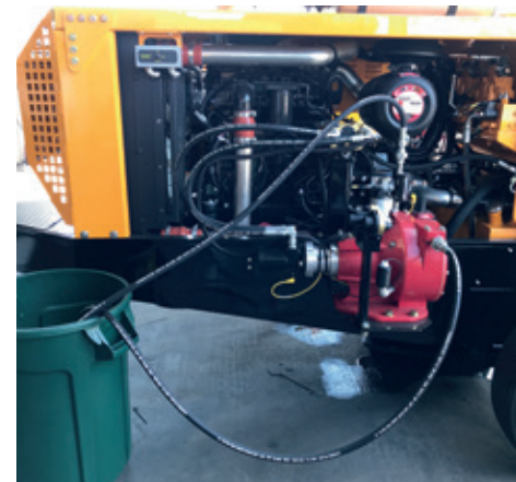
The new fully-synchronised chemical wet shotcrete dosing system from Reed
