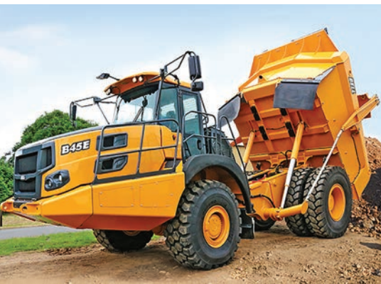
The B45E 4x4 introduces the conceptual advantages of Bell Equipment's two-axle ADT to the 40-tonne payload class
