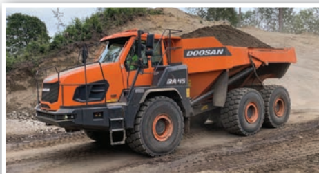
Doosan's DA45-7 Stage V-compliant ADT has a payload capacity of 41 tonnes
