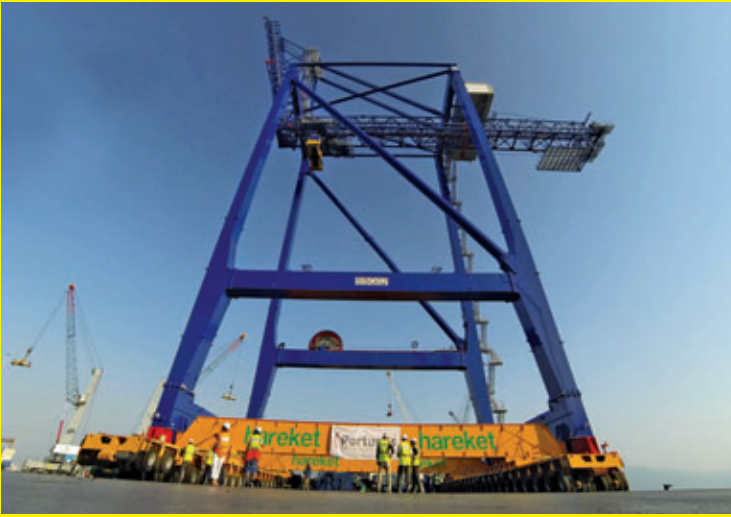
Transportation of 1256 tons Liebherr Port Crane with 2 pcs. 24 axles 2 file Goldhofer PST/SL-E trailer.
