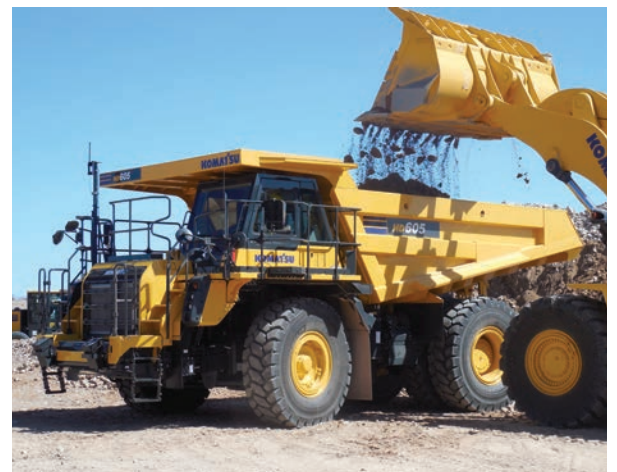
The Komatsu HD465-8 and HD605-8 both feature the Komatsu Traction Control System
