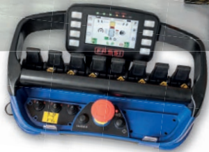
Fassi and Volvo Trucks developed the Drive by Fassi system to remotely operate the truck, at
