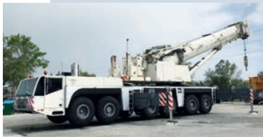
The 350 tonne capacity Demag AC 350 has a 64 metre boom and a six axle carrier
