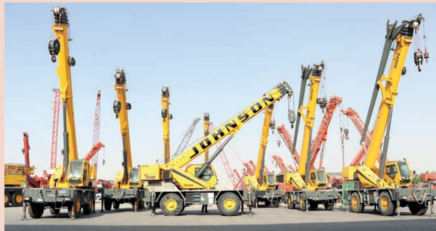
Johnson Arabia displays some of its ten new Grove RT550Es, which can each lift up to 45 tonnes
