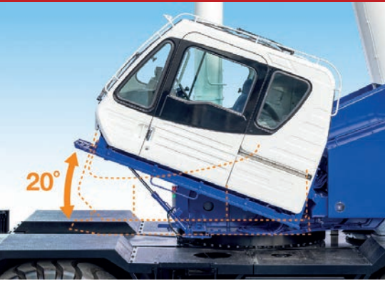
A cab tilting mechanism is now available for Tadano rough terrains
