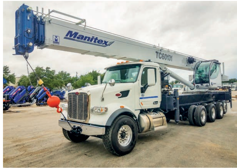
The TC600 is Manitex's newly released boom truck mounted crane with a maximum main boom height of 141 feet (43 metres)
