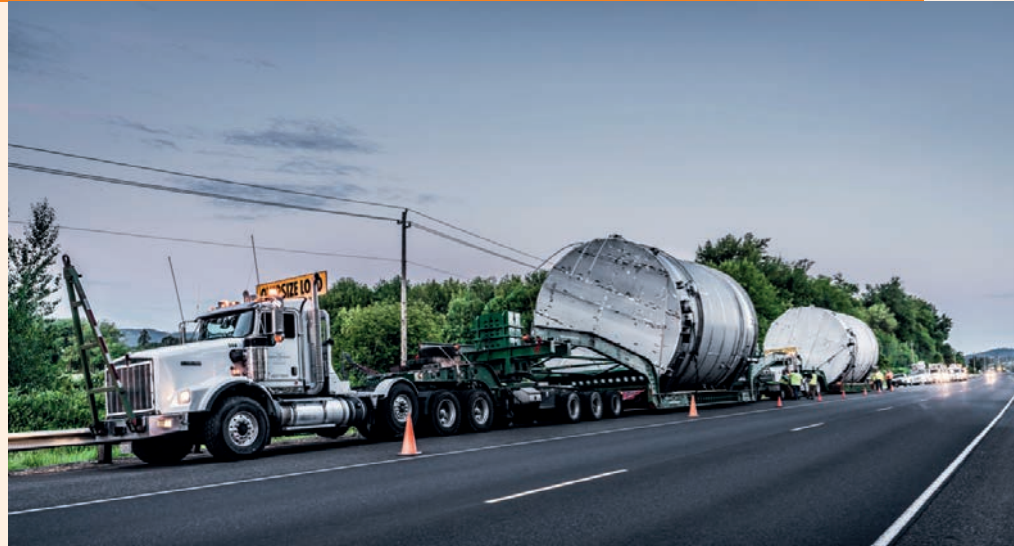
Omega Morgan's innovation centered on solving extreme route challenges, keeping the tight schedule and not modifying or damaging the ozone tanks
