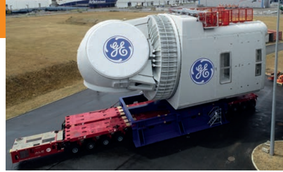
In France ALE used 32 axle lines of SPMT to transport two wind turbine nacelles
