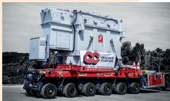
Six axle Cometto MSPE carrying 85 tonnes
