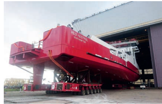
ALE used 36 lines of SPMT to launch a 750 tonne ferry on the River Mersey in north west England
