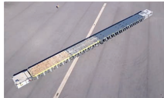
Cometto's SyncBox enables a number of its SPMT to connect with self-propelled vehicles from other manufacturers
