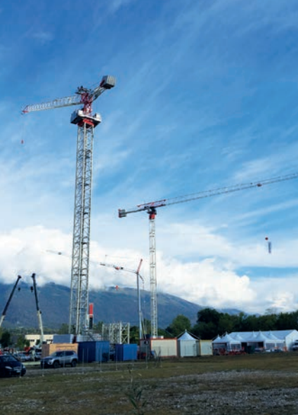
The Terex CTLH 192-12 hydraulic luffer, the CTT 172-8 flat top and the new CSE 32 self erecting tower
