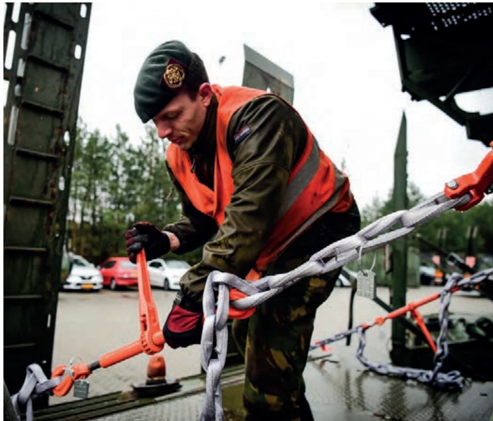
The Dutch NATO defence force has started using synthetic link chain for heavy haulage applications
