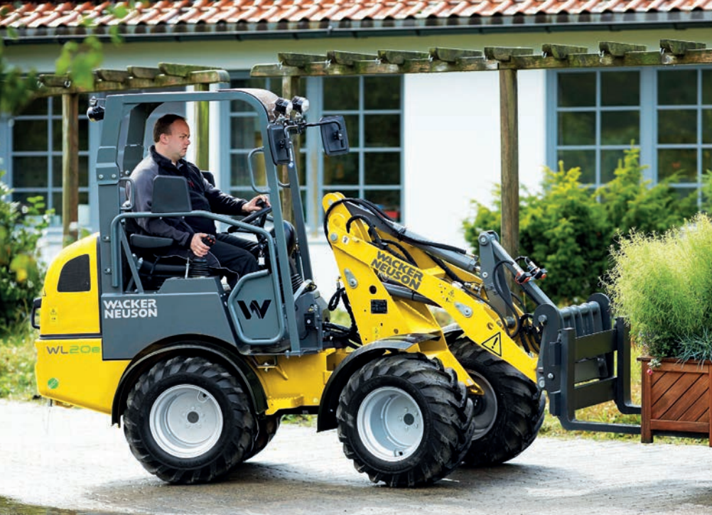
Wacker Neuson's battery-driven WL20e loader, with an absorbent glass mat battery
