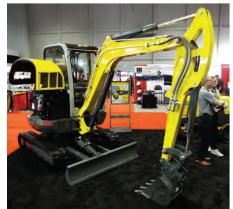
An EZ38 excavator that was reconditioned by Palmer Johnson Power Systems
