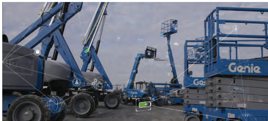
Genie's Lift Connect solution gives equipment owners the ability to see precise machine hours remotely to help manage their long-term maintenance
