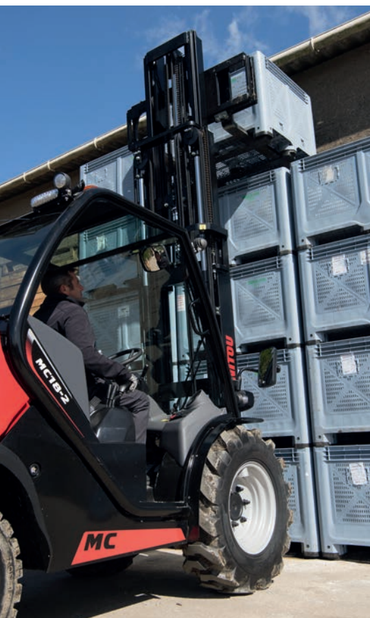
The new Manitou MC18 has an overall width of 1450mm and a height of less than 2m on its Buggy version.
