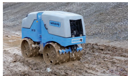
Weber MT's new remote control, Stage V compliant MC 85 trench roller in action
