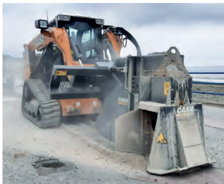
A Case TR270 compact tracked loader with a Case T450 Rock Wheel attachment, being used on the Isle of Man
