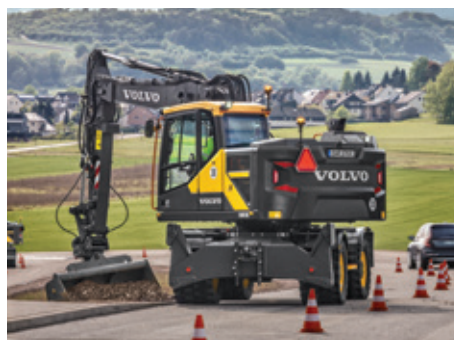
The EWR170E has been designed to meet the growing demand for short swing wheeled excavators
